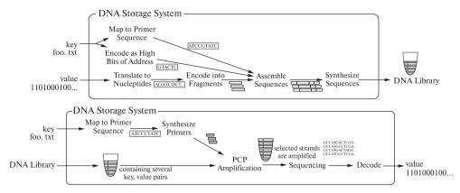
Fig. 3.9. Overview of a DNA storage system [81]
