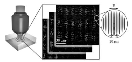
*Fig. 5.16.* 5D optical data storage, written in fused quartz using a femtosecond laser. Three spatial dimensions and two optical ones (the slow-axis orientation and the retardance) are exploited. Each voxel contains a self-assembled nanograting which is oriented in a direction perpendicular to the light polarization [163]
