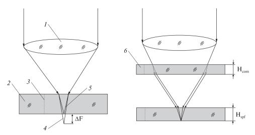
*Fig. 5.26.* Schematic representation of aberration compensation: 1 - objective lens, 2 - sapphire substrate, 3 - optical axis, 4 - extraordinary ray, 5 - ordinary ray, 6 - compensating plate
