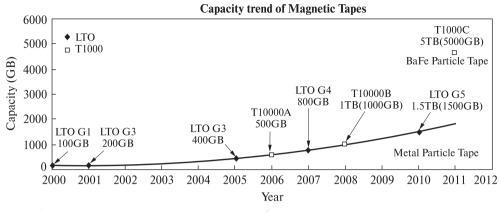
Fig. 3.3. Increasing the capacity of magnetic tapes [61]
