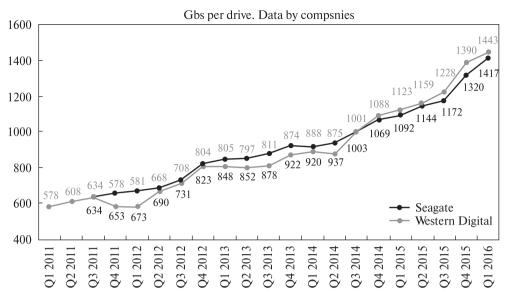
Fig. 3.1. Increase in areal density on hard magnetic disks [52]
