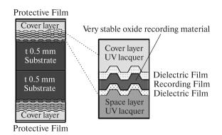
A significant increase in the capacity of Arhival Disc compared to the Blu-ray Disc was achieved by applying multiple technical solutions. By implementing six discrete recording layers (three on each side), the new standard achieves a revolutionary jump in storage capacity, to 300 GB per disc.
