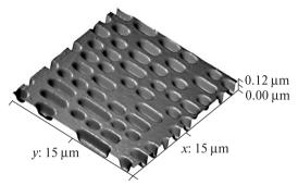
*Fig. 5.30.* General view of sapphire substrate of long-term data storage media
