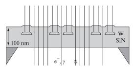
*Fig. 5.8.* W-Si<sub>3</sub>N<sub>4</sub> WORM medium, which is transparent to electron or photon beams [106]
