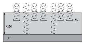
*Fig.* 5.9. W-Si<sub>3</sub>N<sub>4</sub> WORM medium, which is readable by constructive interference on the silicon base and destructive interference on the tungsten islands [107]
