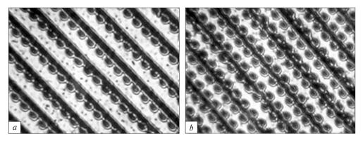
*Fig. 4.8.* External appearance of the recording zone on the optical carrier: data recording is carried out from one side of a guide track (*a*) and from both sides (*b*)
