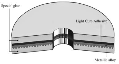
Fig. 5.5. Glass disc for long-term data storage [98]
