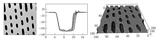
Fig. 5.29. AFM image of sapphire substrate after ion-beam etching
