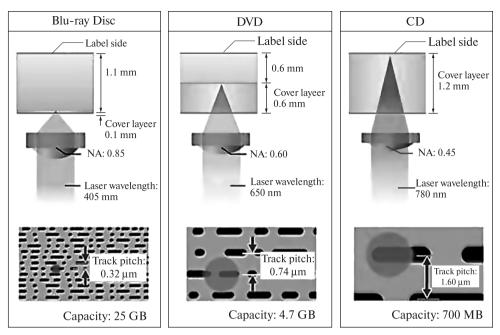
Fig. 4.1. Improving the systems of optical information recording [89]
