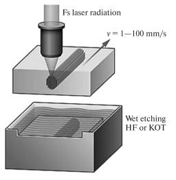
rial is transparent at lower intensities. Therefore, laser radiation with pulse duration of picoseconds or shorter and focusing to a few microns is necessary. The material is heated by the absorbed energy during a short time to high temperatures, resulting in large local pressures. Because only a volume of several cubic microns is heated, the material cools rapidly and is quenched in a modified state. For example, single
