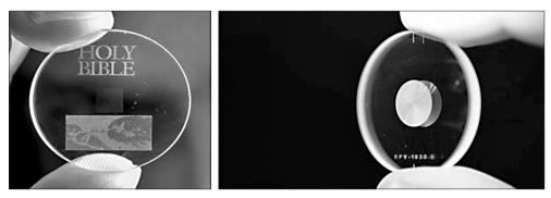
Fig. 5.18. Appearance of fused silica media for long-term storage [172]
