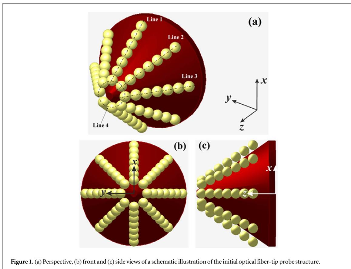
**Figure 1.** (a) Perspective, (b) front and (c) side views of a schematic illustration of the initial optical fiber-tip probe structure.
